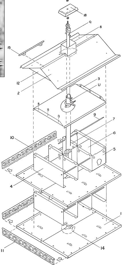
Make *sure* parts are in correct location before bending tabs.
