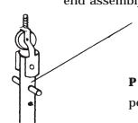
**P 5.** Install 1/4x2 split pin [H] in second hole below pulley in post top section [Q]. Drive pin through post until centered.
