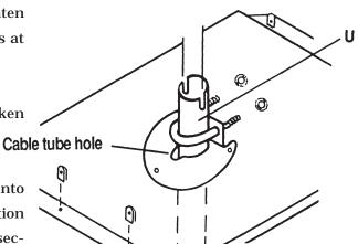
**17.** Thread cable through chimney from underside of roof. Attach roof to ceiling as shown with six 6-32x3/8 PHMS [24]. Flat 'C' nuts can be positioned with a small nail if required. Roof is on outside on both ends.
