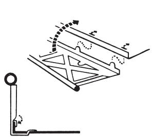
**9.** Fasten chimney [8] to **one** roof section [2] using two 6-32x3/8 PHMS [24] and two 6-32 acorn nuts [23]. Do not tighten screws until assembly is completed.
