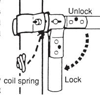
**P 3.** If handle is not locking tight, turn nut 1/2 turn tighter; if too coil spring tight, loosen 1/2 turn. Raising
